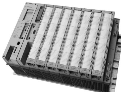
Figura No. 5. PLC Siemens Simatic S5
