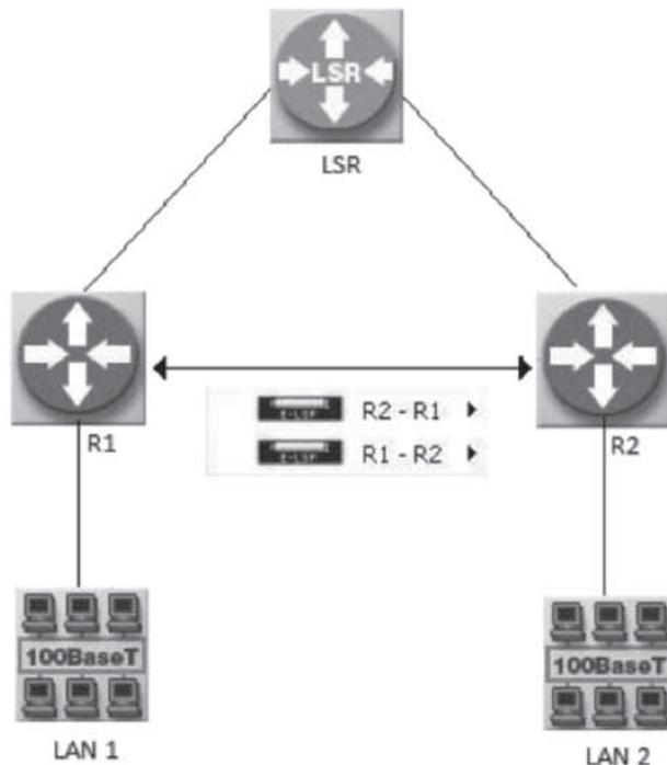
*Figure 1. Schematic of the simulated network for comparing the various queuing algorithms.*
