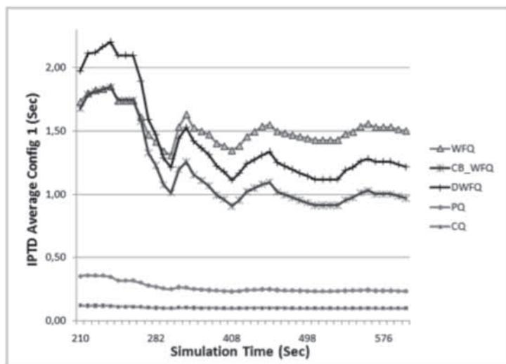
Figure 2. IPTD parameter for the simulated queuing mechanisms. ( Cuéllar & Navarro, 2010c ).
