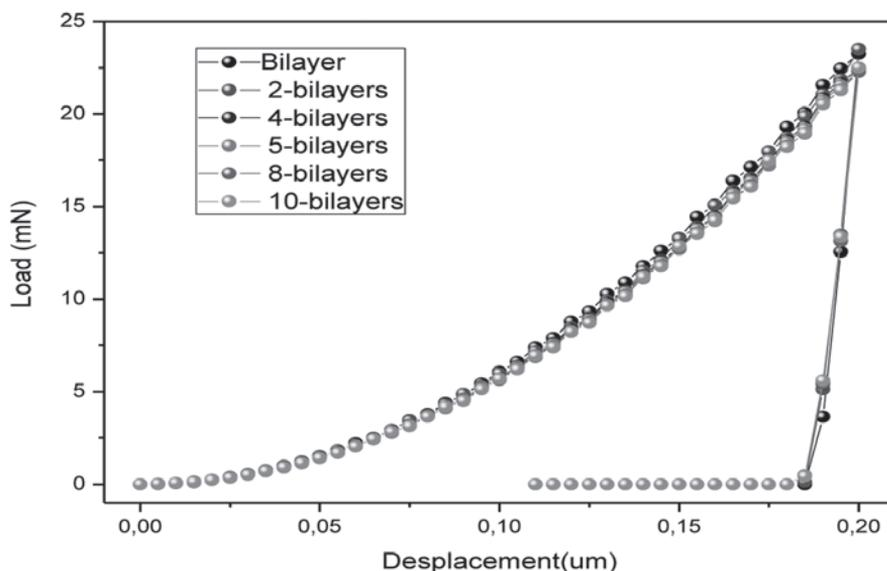
Figure 2 Load-displacement curve during indentation loading and unloading as a function of the number of bilayers
