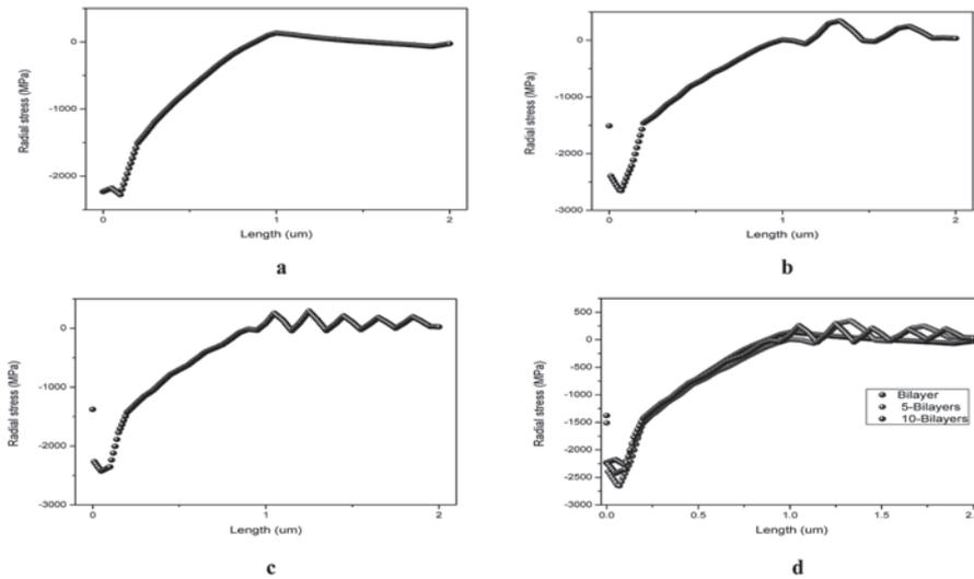
Figure 4 Curves of radial stress (a)1 bilayer, (b) 5 bilayers, (c) 10 bilayers, (d) overall
