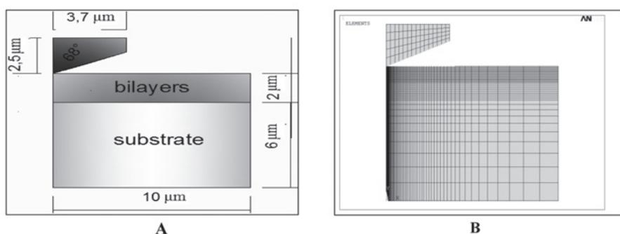
Figure 1 (a) Substrate-bilayer system and indenter size and
